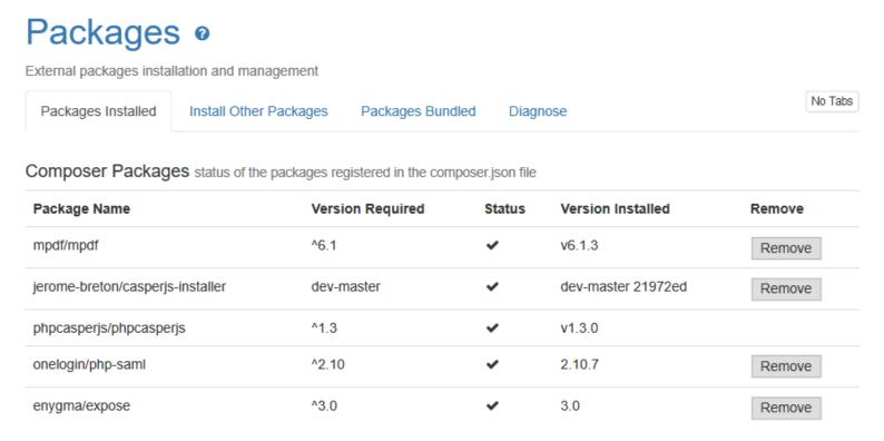
The status column shows a success icon ( $\checkmark$ ) if the package is installed, or a warning icon ( $\triangle$ ) if it is missing. If the package is missing, you can click the "Fix Missing Packages" button that is displayed and Tiki will try to install the package again.
